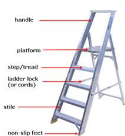
Figure 14: Most important parts of a platform ladder
